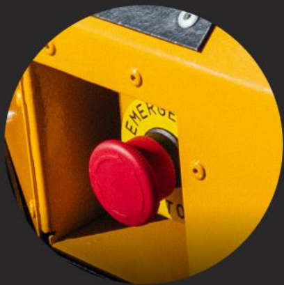
Platform power emergency stop button
