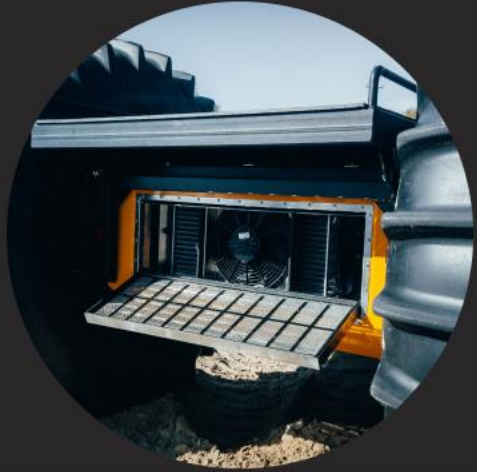
Access to radiator fan and replaceable mesh filters
